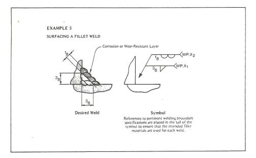
The same Example may be used to illustrate the application of a surfacing symbol for the purpose of increasing the size of the fillet. In such case, however, the size of the surfacing weld will have to be calculated from the increment in the leg size as required for the new fillet weld.
