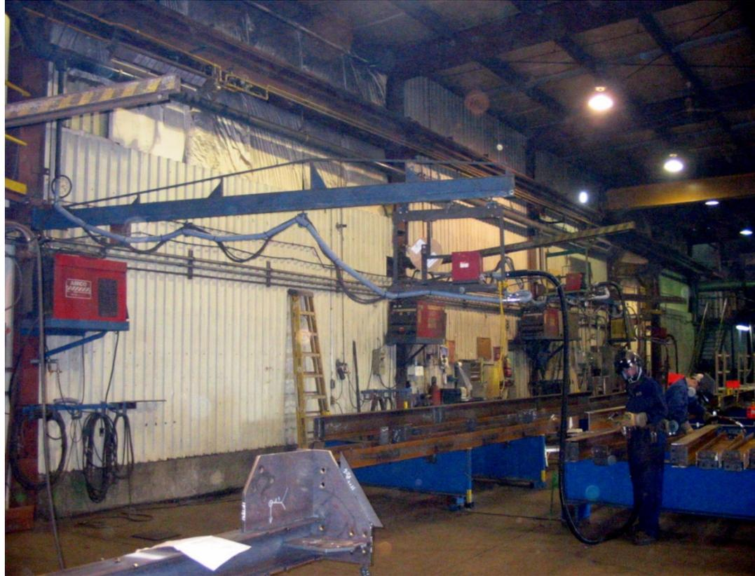
**Smoke extraction welding gun installed on wire feeder mounted with a long reach jib, rotating on a vertical axe at the building column.**
