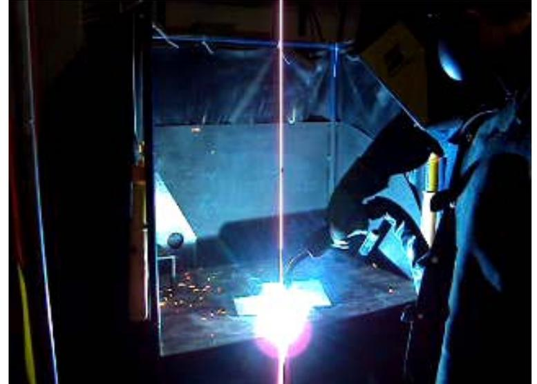
**Arc-Air gauging process into an enclosure that has 2 doors on each of the 4 sides where the operator works from.**
