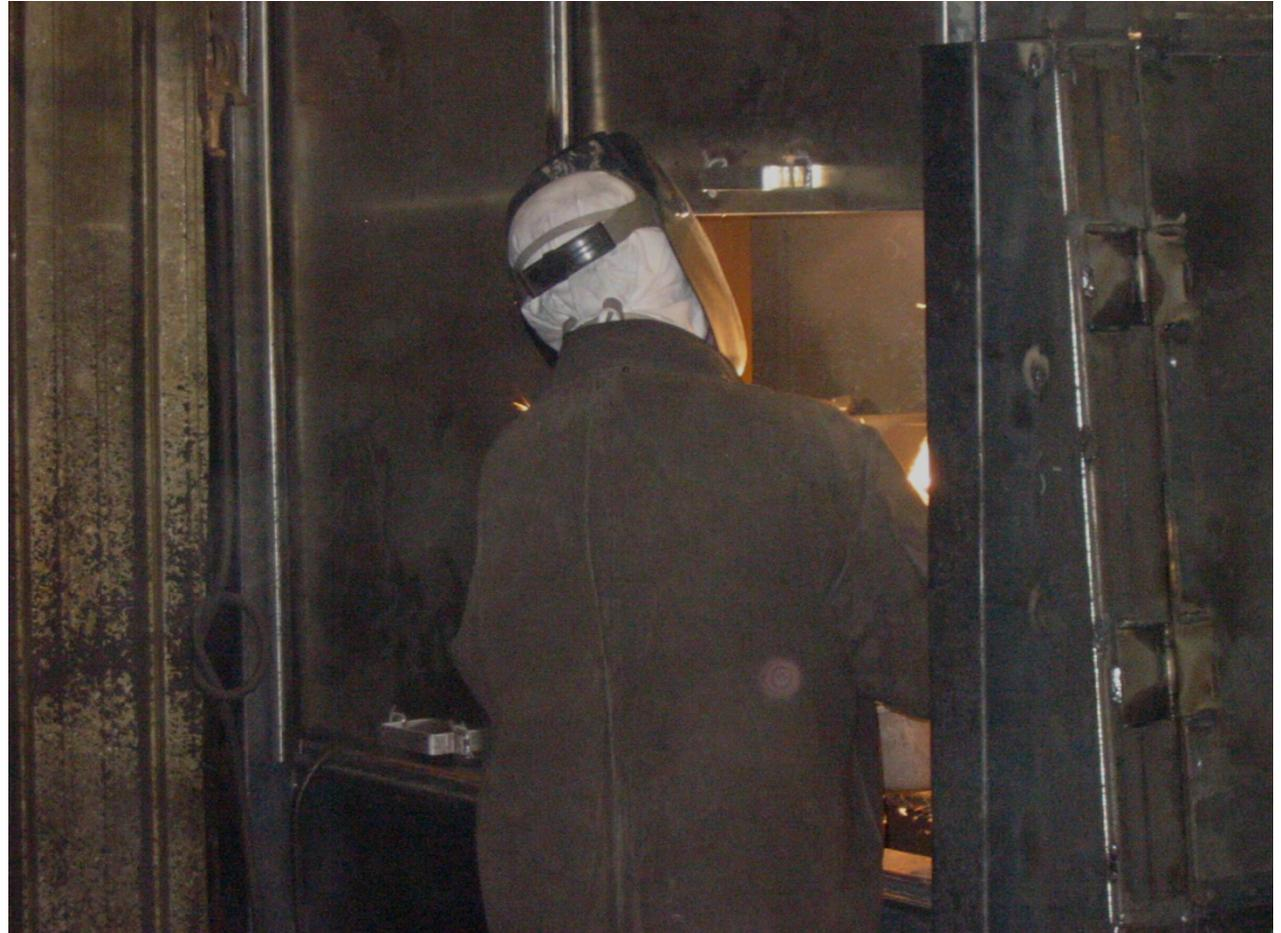
**Only the operator's arm is in the contaminated space of the enclosure.**
