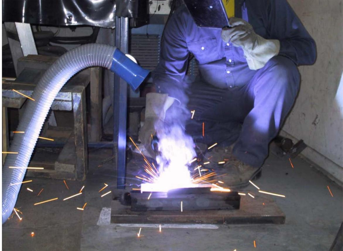
**3" flexible pipe with a 3 inch capture hood in position with a magnet.
