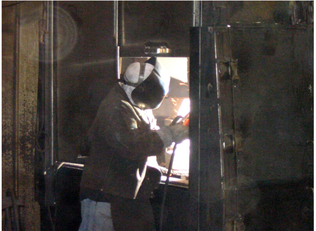
**The operator does not inhale air contaminated by the gauging process.**
