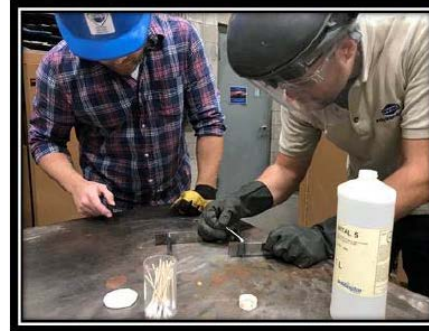
Welder certification is subject to different forms of destructive testing such as fracture and macro etching (above) and the guided bend test (below)
