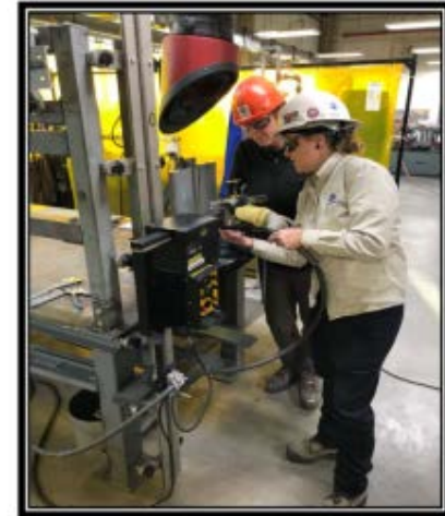
Welding instructor Jackie Hache teaches the operation of the oscillating attachment on the BUG-O
