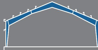
Clearspan with tapered columns
